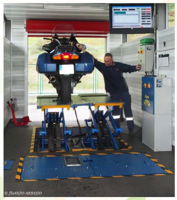
Special line for Motorcycles PTI / Picture co<mark>urtesy of</mark> itvasa of its facili<mark>ties</mark>
