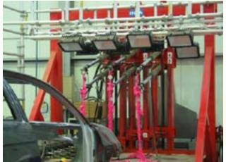
Testing machine for seat anchorages © INTA - Spain
