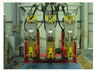
Testing machine for safety belt anchorages © INTA- Spain
