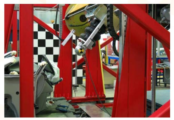
Testing machine for head impact © INTA - Spain
